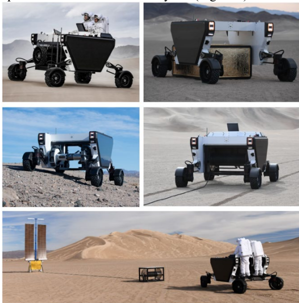
Figure 1: FLEX's modular payload interface and novel mobility system enable it to perform a multitude of functions, including (left to right, top to bottom): crew transport, outpost logistics, robotic science, and infrastructure deployment
