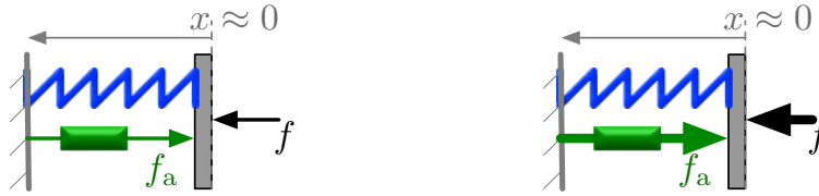
Figure 5.12: The force sensor operated using the force-balance principle. The deflection x is sensed, and is fed back to produce the actuator force f_a required to counteract the externally applied force f so displacement is kept at zero x \approx 0 . This required actuator force is then the measurement of the externally applied force. In this manner, the sensor is always operating in the linear regime shown in Figure 5.11, which is the regime of highest sensitivity. When operated in this manner, the force-balance sensor has much higher sensitivity over a large dynamic range.
