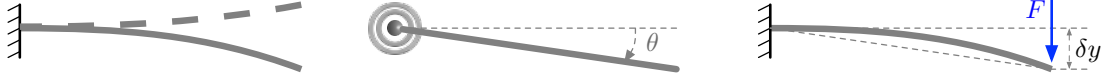
Figure 1.20: (Left) A full model of the vibrations of a clamped-free beam requires using a partial differential equation to solve for the “modes” of vibration. Here, the first such mode is depicted. (Middle) A simplified approximate model for a clamped-free beam is as a rigid beam pivoting around a torsional spring. (Right) To determine the effective torsional spring constant, we can use the static deflection equation for a clamped-free beam which states that the deflection \delta y = \frac{L^3}{3EI} F , where F is the force applied at the free end. The effective torsional spring constant is then obtained from the ratio of applied static moment FL to the resultant static angular deflection \delta\theta \approx \delta y/L , i.e. k_{\text{eff}} = \frac{FL}{\delta\theta} \approx \frac{FL}{\delta y/L} = 3EI/L .
