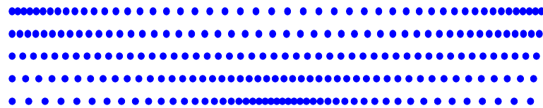
(c) The second normal mode begins with a compression wave either in the middle or at both edges. The compression then propagates from one configuration to the other repeatedly. The diagram depicts 1/2 of a period. Click for animation . See also the 3rd mode animation , the 4th mode animation , as well as the animation of the first 4 modes together .
