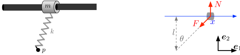
Figure 1.9: Example 1.5: A mass restricted to move without friction on a linear guide. The mass is connected with a spring to a fixed pivot point as shown. While the mass' motion is restricted to be one dimensional, the spring force is a vector in 2D whose direction varies with x . The motion along the guide is governed by the component of the spring force parallel to the guide.
