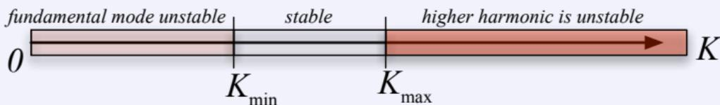
*Observation:* Which higher harmonic becomes unstable at high gain (e.g. 3<sup>rd</sup> or 5<sup>th</sup>, ..) depends on mic placement!
