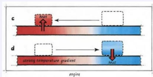
Similar principle as “pulse-tube refrigerators”
