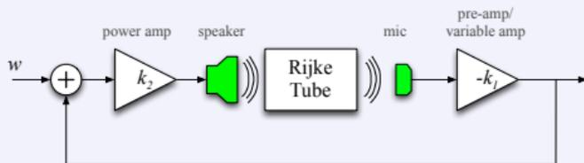
With simple *proportional acoustic feedback*  $K$ , can stabilize this system!
