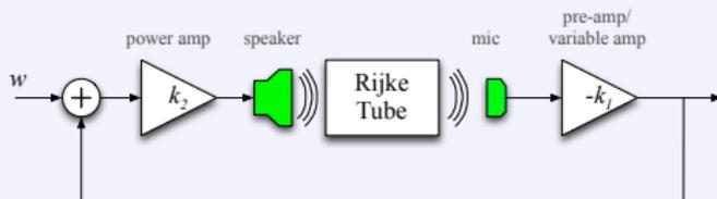
With simple *proportional acoustic feedback*  $K$ , can stabilize this system!
