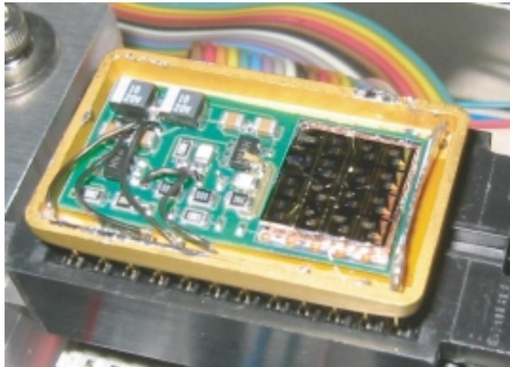
Figure A.2: Picture showing the PCB and the cantilever die during testing.
