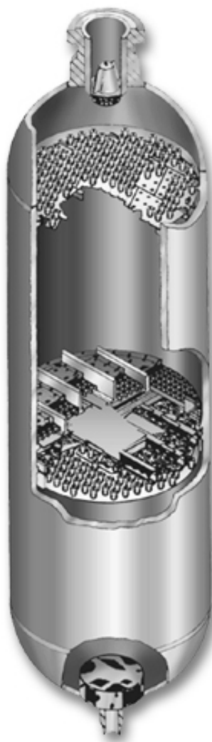
Figure 1.14: Expanded view of a multibed HDS reactor showing the gas distribution tray at the top and the catalyst support tray in the middle; these reactors can range in diameter from 1.5–5 m. Courtesy of UOP LLC.
