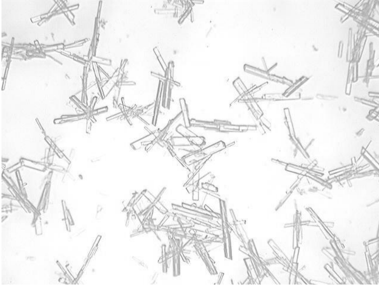
Figure 10.3: Growing pharmaceutical drug crystals with a needle-like particle shape. Images taken after particles have settled on a microscope stage.
