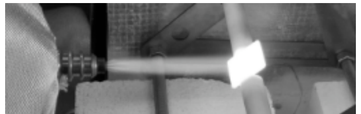
Figure 6: R512E-coated C103 in H_2+O_2 torch setup
