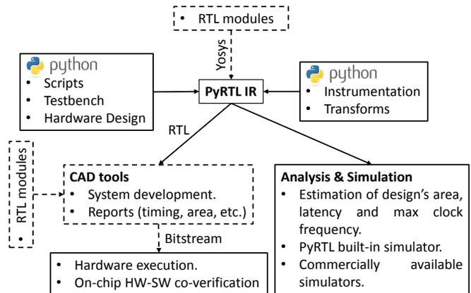
Fig. 1. Overview of PyRTL’s flow.
