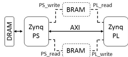
Fig. 6. System architecture.
