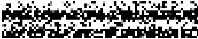
Fig. 1: Distribution of startup probabilities in a sample section of an SRAM. The black pixels always resolve to a 1, while the white pixels always resolve to a 0. The grey pixels have a probability between 0 and 100, with the depth of color reflecting the probability. A pattern of alternating regions of bias were present in all tested memories.
