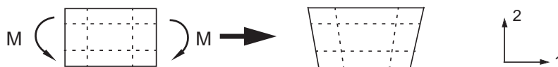
Figure 4–5 Deformation of a fully integrated, linear element subjected to bending moment M .
